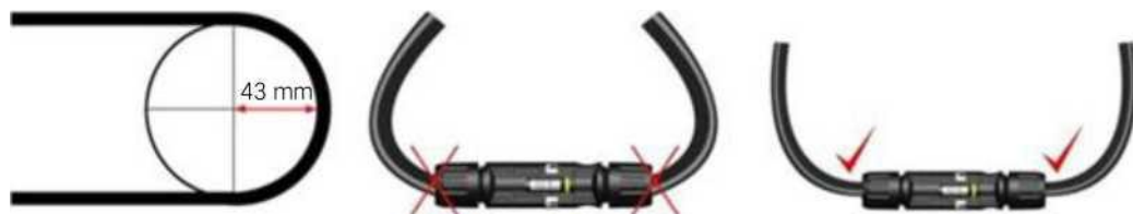
The correct routing and minimum bending radius of cables.
